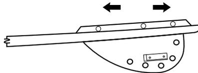
A horizontal adjustment forward (toward the tip of the ski) lifts the front and drops the tail during an on-side turn. A horizontal adjustment backward drives the front into the water and raises the tail.
